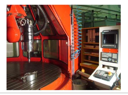
Machine tool: Hybrid parallel kinematic structure
