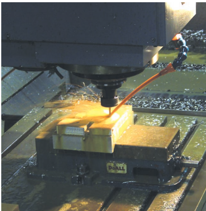
A machine tool can receive STEP-NC data, "understand" what it means and begin milling without any more instructions.
