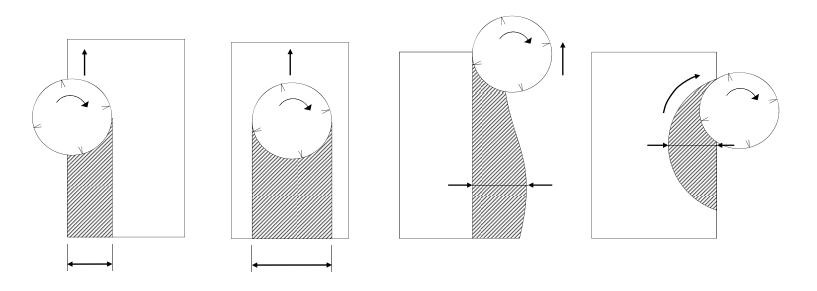
$\mathcal{C}_r$  = Radial Depth of Cut / Cutter Diameter
