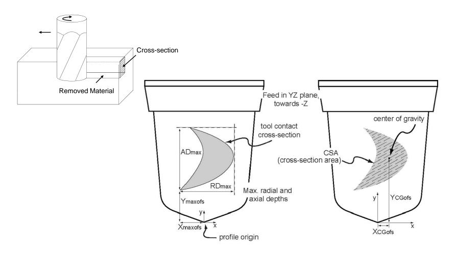
Figure 34 - Cross-section parameters for milling
