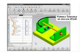
Figure 3 - Assembly tolerances
